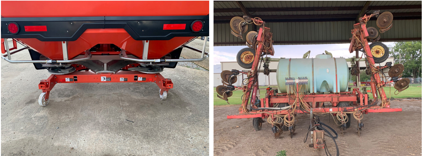
Figure 1. Application equipment included a granular applicator (left) and liquid knife applicator (right). The liquid surface applied applicator is not shown.
